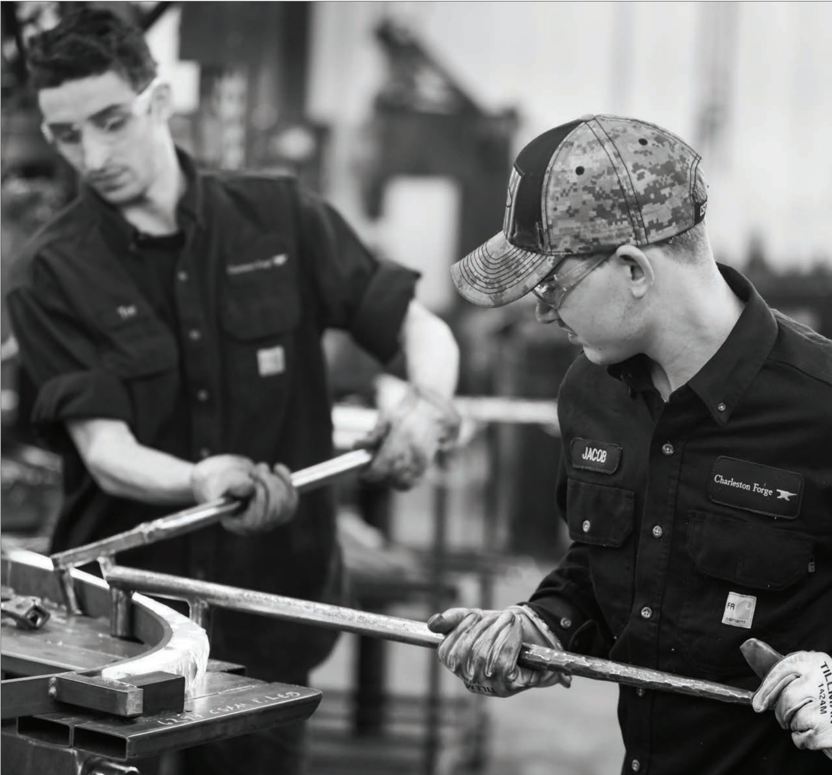
Forgers use a jig while bending the leg of a Triumph Dining Table. Jigs ensure that bends are consistent which means we deliver a perfectly symmetrical and level product every time.
